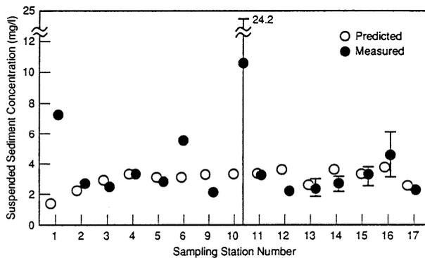
Fig. 3. Predicted total suspended sediment (sum of sand, silt and clay) Concentrations
